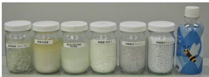
The stages of recycling PET resin, from the initial PET flakes (far left) to the final PET bottle (far right)
